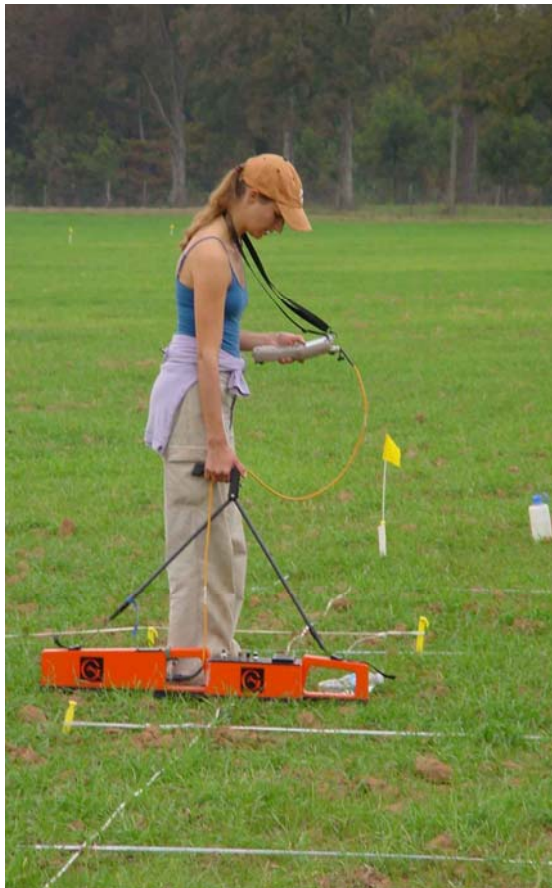
Kattie Simon, a volunteer and member of Ken Kvamme's remote sensing class, using the Geonics EM38 conductivity meter at Battle Mounds. Photo by Anthony Clay Newton.
