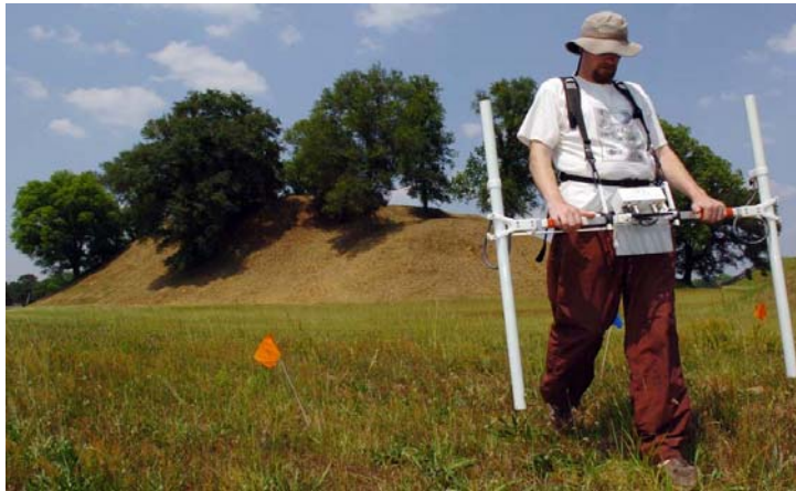
University of Arkansas graduate student Duncan McKinnon using Bartington 601 Fluxgate Magnetometer to look beneath the surface without digging at Etowah Mounds in Georgia. Duncan will be doing similar work at Battle Mounds this fall.
