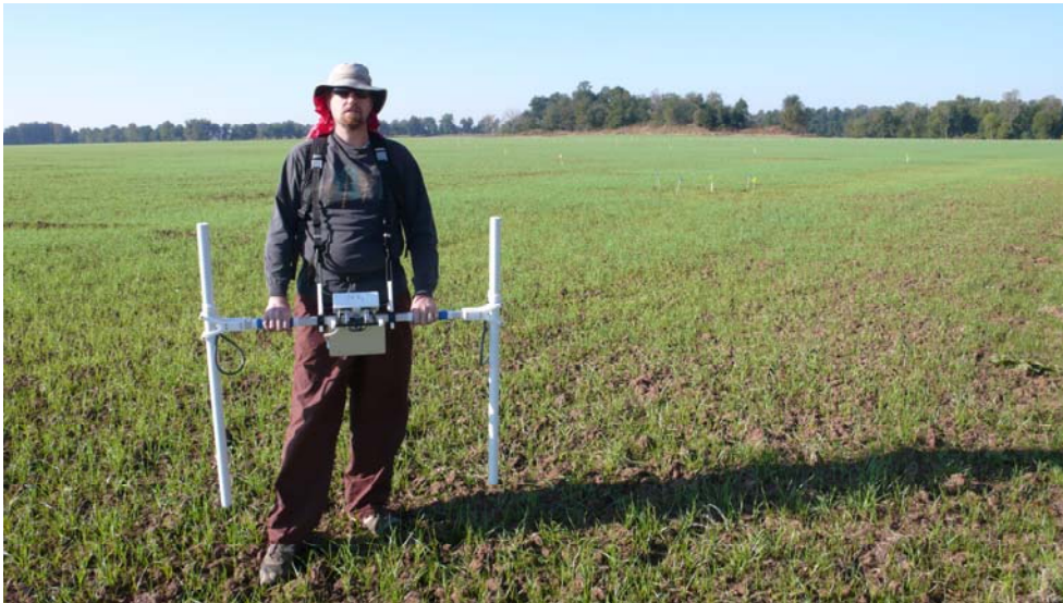
Duncan McKinnon with the Bartington 601 Fluxgate Magnetometer in front of Battle Mound (on the horizon) last fall. We have surveyed 200 20 x 20 meter grids of the site with geophysical equipment—that’s 80,000 square meters or almost 20 acres. Photo by Anthony Clay Newton.
